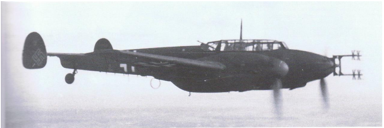
Above: Bf 110F-4a of III./NJG 1 with four nose-mounted FuG 202 Lichtenstein BC radar antennae, each with four dipoles and four reflectors used jointly for transmission and reception, flown by Fw 'Teddy' Kleinhenz and his Bordfunke r, Uffz Hermann Gampe, from Leeuwarden, Holland, February-April 1942. (via Theo Boiten)
