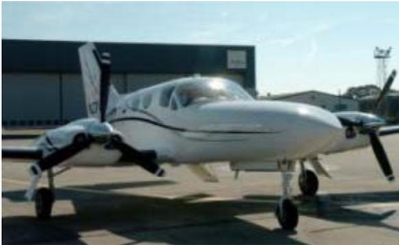
**N37VB** is a 1978 Cessna 421C, a 6-8 seat pressurised low-wing monoplane powered by two 375hp Continental GTSIO520 turbocharged piston engines. Its maximum take-off weight is 3.4tons and it carries 1400lbs of avgas fuel.
